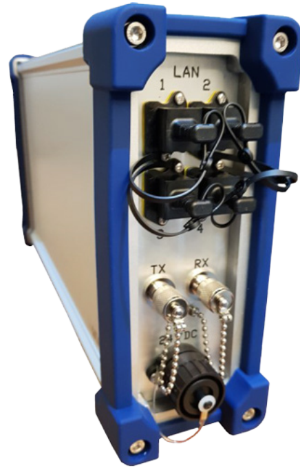
Rear of Q-Lite Rugged modem showing weatherproof connectors (4 x Ethernet, Tx, Rx and DC input). A mounting bracket allows the modem to be secured in place. Several mounting options are available and can be customised to suit individual requirements.
